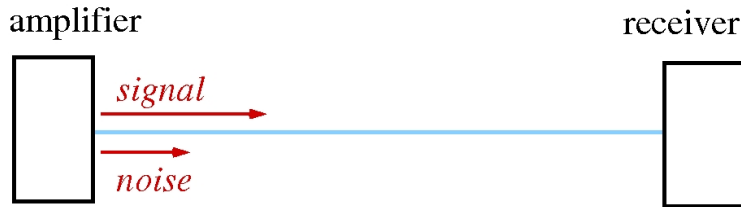
Figure 2: Noise is mixed into the signal as the signal is reinforced at every amplifier along its path.
