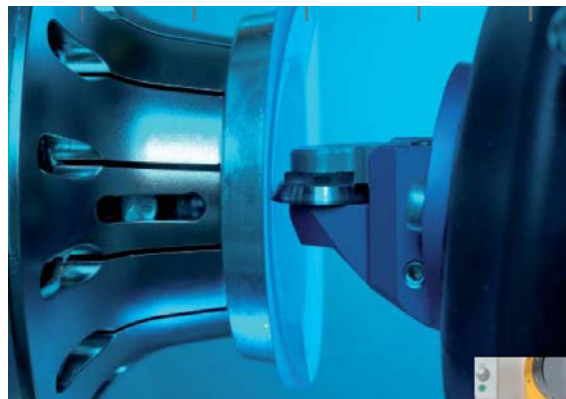
figure 1 Lens surfacing by a lathing tool
