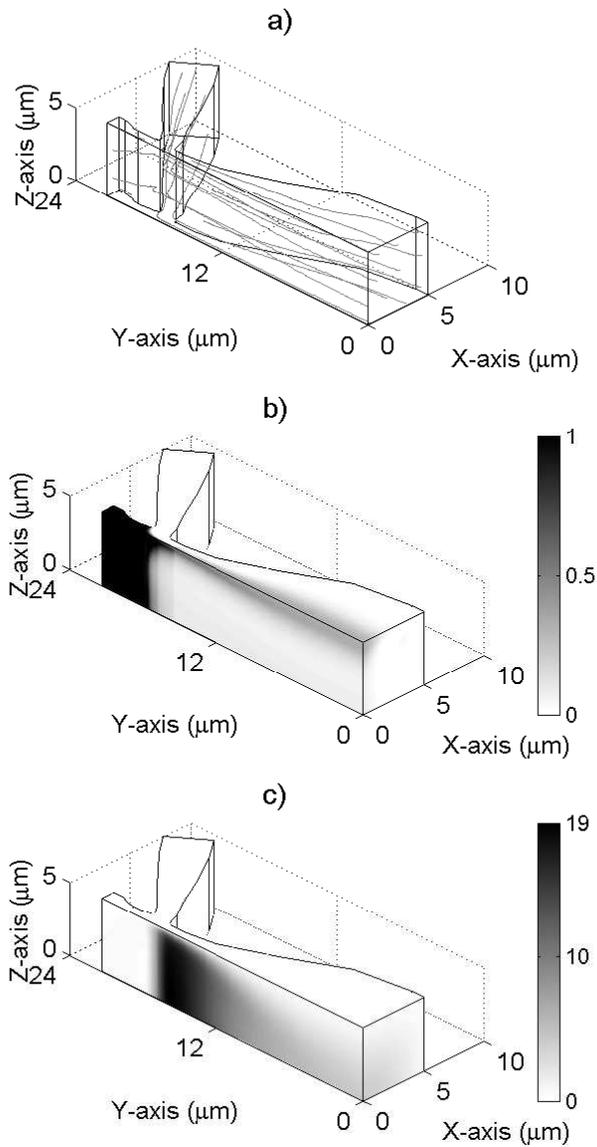
Figure 7: Sample results from the optimized mixer design as simulated with the 3D model. Shown are isometric views of the shape of the optimized mixer with representation of **a)** selected streamlines generated by considering the velocity field, **b)** the concentration distribution, and **c)** the velocity amplitude distribution.
