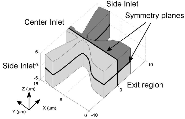
Figure 1: Typical domain representation of the microfluidic mixer geometry considering the 3D model: in dark gray we represent the domain  $\Omega_{3D,s}$  used for numerical simulations. The geometry's symmetry planes are highlighted and labeled.
