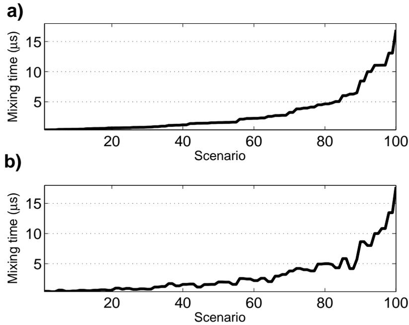
Figure 3: Mixing times of the 100 microfluidic mixers (called Scenarios), randomly generated during the 2D versus 3D comparison process and sorted considering the 2D mixing time, as computed when considering **a)** the 2D model and **b)** the 3D model.
