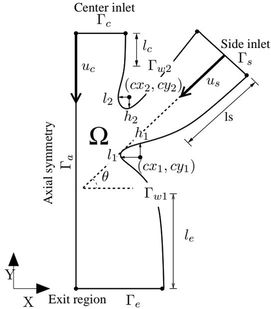
Figure 2: Typical representation of the domain  $\Omega_{2D,s}$  and parameterization of the microfluidic mixer considered for the optimization process.
