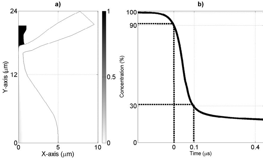
Figure 5: Optimized mixer simulated with the 2D model: **a)** shape of the optimized mixer with a superposed color plot of the denaturant concentration distribution and **b)** the time evolution of the denaturant concentration of a particle in the symmetry streamline.
