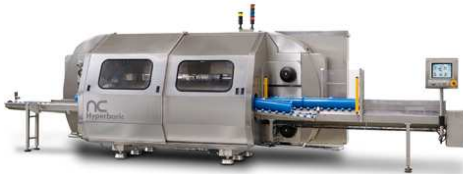
Figure 5.1: Example of horizontal, large commercial HPP vessel. Model Hiperbaric 55. Hiperbaric, Burgos, Spain. [42]
